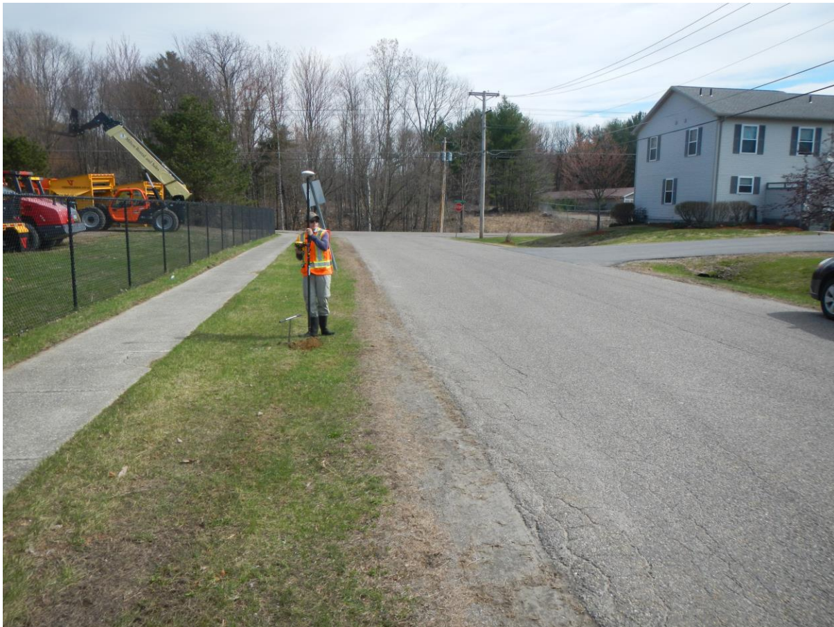
Figure 4: FEA staff collecting survey data and soils data for a grassed swale BMP along Nancy Drive (Project RT7-16)
