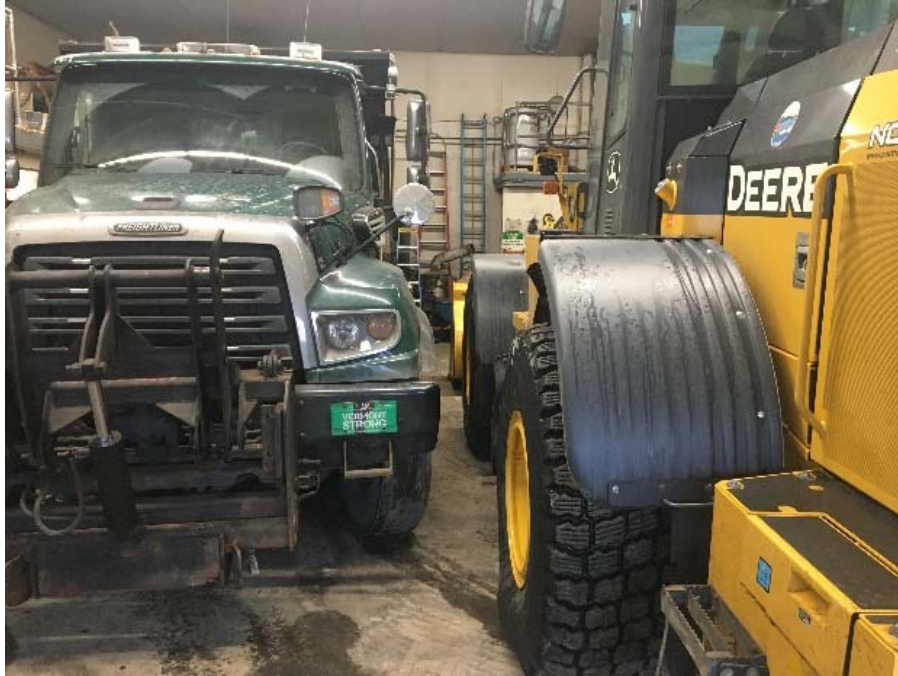
Photo 1. Proximity of vehicles stored during freezing overnight conditions. No room for staff to walk between vehicles.
