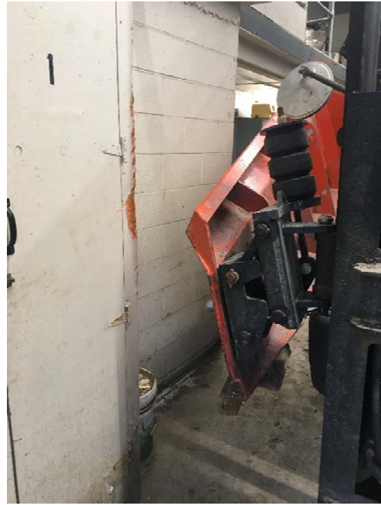
Photos 3 and 4. Plow wings within inches of the wall.
