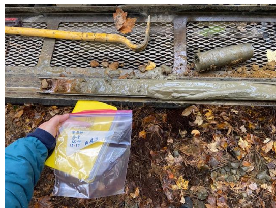
Very loose, wet Lacustrine & Marine Silt
