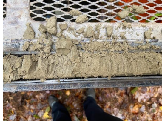
Poorly graded sand and silt above the Lacustrine & Marine Silt
