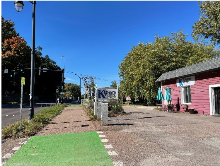
Photo 24: Riverside Avenue shared use path in Burlington with green paint at intersections with driveways (Source: VHB)
